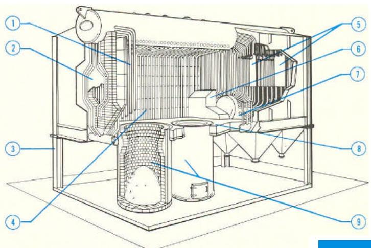
Fig. "A": 25,000 pph Wood-Fired "VL" with Air-cooled Pin Hole Grate
